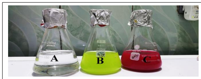
Figure (1): The change in the color of Photosynthesized Selenium Nanoparticles using Aas ( Myrtus communis L.) Leaves Extract, A, Sodium selenite solution. B, Aas ( Myrtus communis L.) Leaf Extract. C. Photosynthesized Selenium Nanoparticles colloidal.
