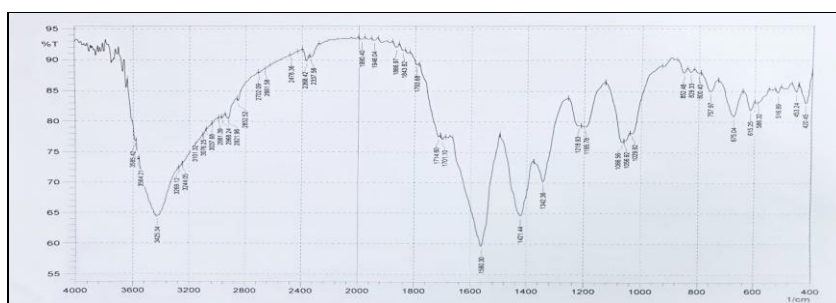
Figure (4): FT-IR spectra of Photosynthesized Selenium Nanoparticles using Aas ( Myrtus communis L.) leaves extract (MC-SeNPs).
