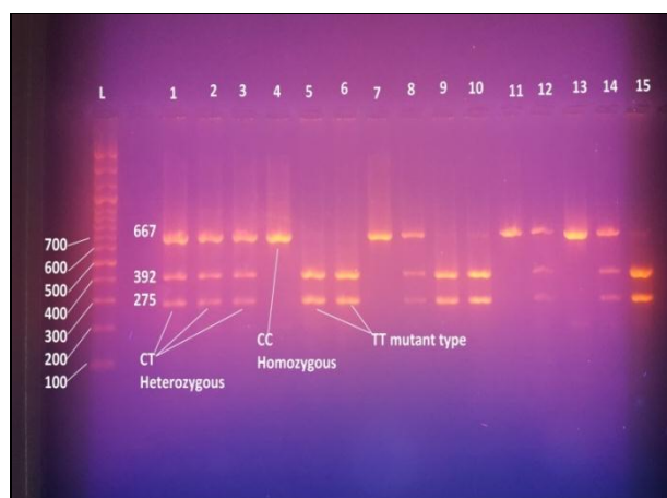
Figure (3): PCR product treated with Cci I electrophoresis on 3% concentration. Agarose gel at 70 voltages for 90 minute. The product of (RFLP) were Visualized under U.V light after stain with
