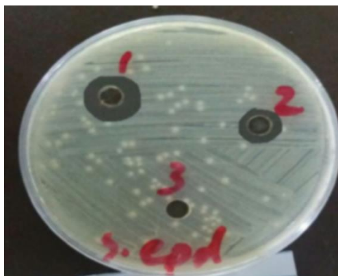
Figure (8): Inhibition Zone of ZnO NPS prepared by (1) Irradiation method (2) precipitate method for S. epidermidis (3) solvent (D.W).
