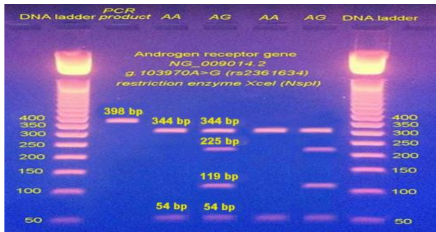
Figure (8): PCR product (398 bp fragment) in intron 1 of androgen receptor gene digested with NspI restriction enzyme and electrophoresed on 2% agarose. The genotypes at 103970 position (NG_009014.2) are: AA (54 and 344 bp), AG (54, 119, 225 and 344 bp) and GG (54, 119 and 225 bp).
